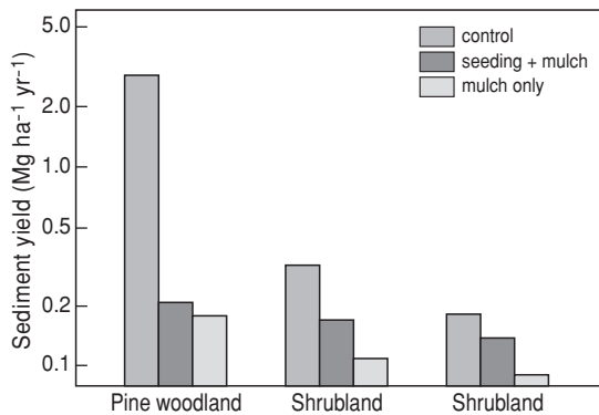
Fig. 14.3 Total sediment yield ( \text{Mg ha}^{-1} \text{yr}^{-1} ; log scale) in three different burned slopes (one pine woodland and two shrublands) in Benidorm, south-eastern Spain, subject to three different treatments: control (untreated), mulch only ( 200 \text{ g m}^{-2} of straw) and mulch plus seeding (grasses and legumes). The area was burned in August 1992 and the sediment yield was recorded from May 1993 to November 1994. Elaborated from Bautista et al. (1996).
